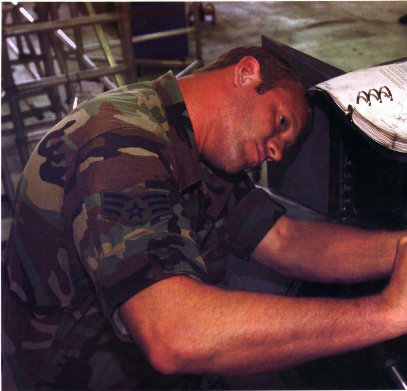
F-15 crew chief SrA. Brian Miller from the 1st Equipment Maintenance Squadron, Langley AFB, Va. tightens retaining bolts on an F-15 rudder actuator.
